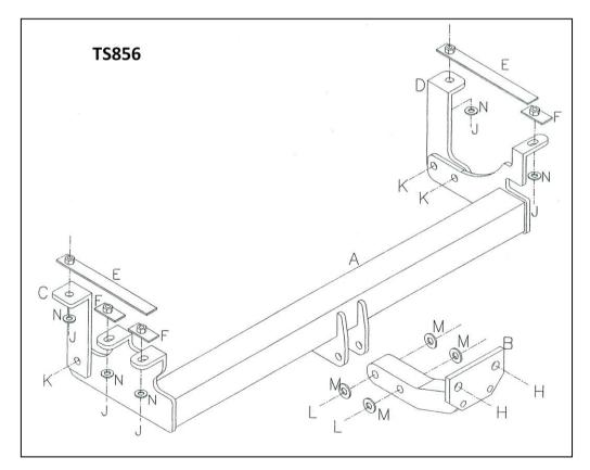
Note: 1. Recommended Torque Setting for M12 Grade 10.9 -139 Nm. (For other Torque Settings see notes overleaf.)
