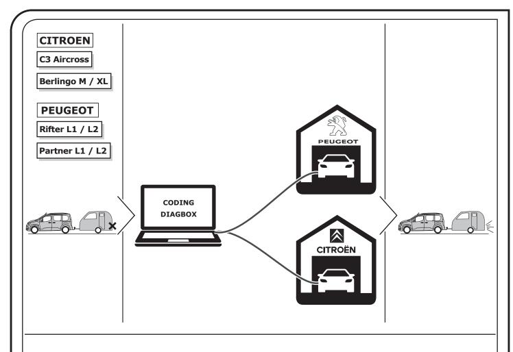
The activation of the trailer functions has to be carried out using the CITROËN DIAGBOX as follows:
